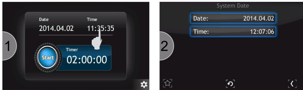
Figure 3.41: Entering system date
