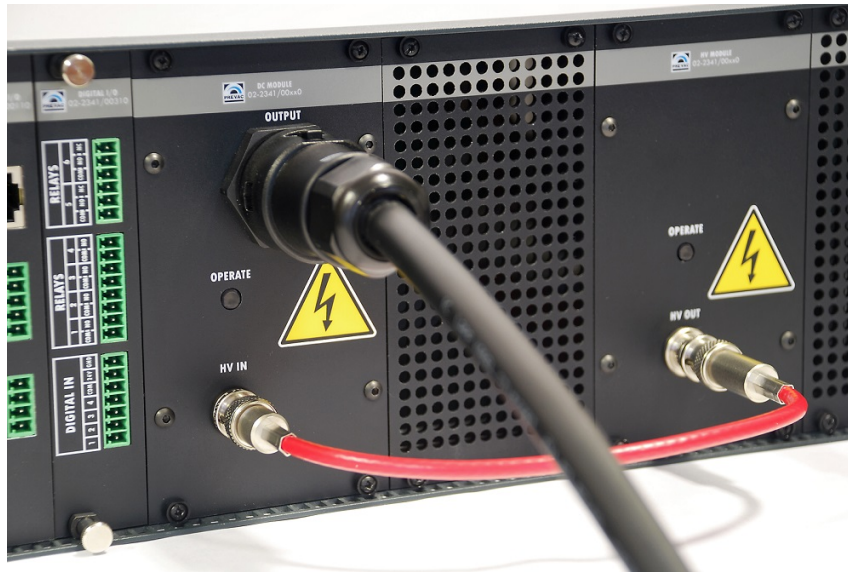
Figure 2.9: Connection necessary for proper operation in Electron Bombardment mode
