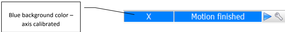
Fig. 17 Calibrated axis motion control panel
