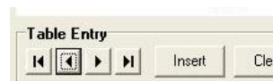
Figure 32. The navigation buttons in the Table Entry section of the Voltage Calibration dialog.
